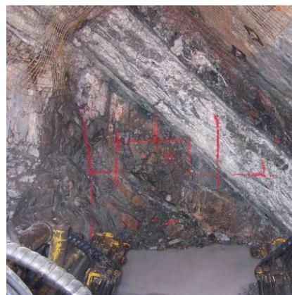
ABOVE: Underground, the gold reef is clearly visible running at a 45-degree angle in lighter colour.
