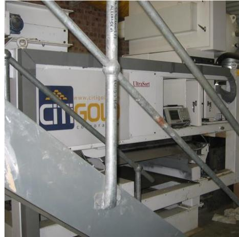
ABOVE: Charters Towers ore from Citigold test mining previously undergoing early-stage 'ore sorting' test trials. The aim is to mechanically remove unmineralised bulk rock 'dilution' that occurs in the ore mining process and reduce tonnage before it enters the wet end of the processing plant.
