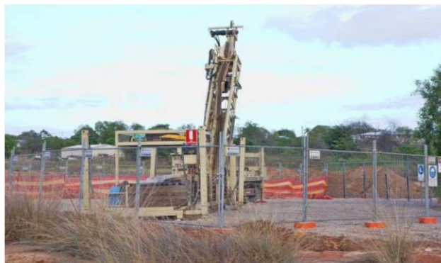
Diamond drill pad drilling the ore body in the Central Mining Area
