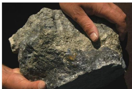
The Charters Towers reefs are physically very different from the surrounding host rock (fine particle granite) and the high grade gold areas within the reef structures contain large amounts of sulphides (iron and lead). The sulphides are a 'proxy' for the gold and silver. The geophysics techniques, which are conducted from both surface and the underground, have shown that they can clearly map the reef structures. Current work aims to refine the sulphide mapping techniques.
